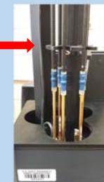
Versa Labs VSM with 6 sample auto-changer
