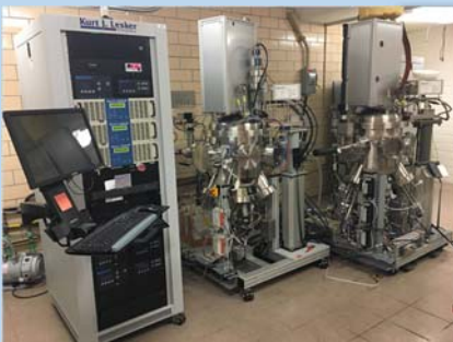
KJLC DC/RF magnetron 3 and 6 gun sputtering systems
