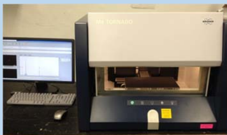
Bruker μ-XRF with 30 micron spot size
